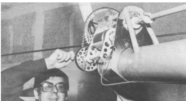
Bob Boucher, consultant for solar cells and electric motor, fits Astro Flight motor. Lower rubber belt cog drives bicycle chain and sprocket to give 23-1 reduction to the propeller.
