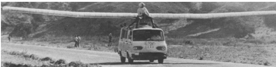
Flat-topped surfaces, unique tail trim, V-P propeller and outstanding structure technique. make Solar Challenger an aerodynamic marvel of the 80s.
