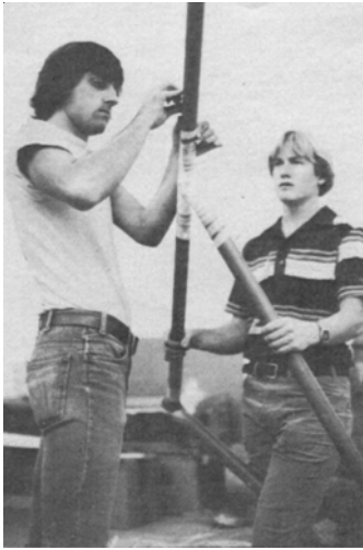
Left: hang glider flyer Carlos Miralles (left) and model flyer Bobby Curtin. assemble fuselage frame tubes: junctions are well reinforced with extra Kevlar cloth and epoxy. Below: Blaine Rawdon, member of Cross Channel Albatross crew, was responsible for most of the structural design on Solar Challenger, seen here on the tube wrapping machine strapping with Tedlar
