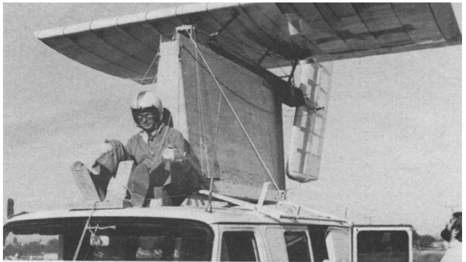
Paul MacCready sits on top of van during 65mph trials to check structural integrity and flutter. Working elevator and rudder operated during tests.
