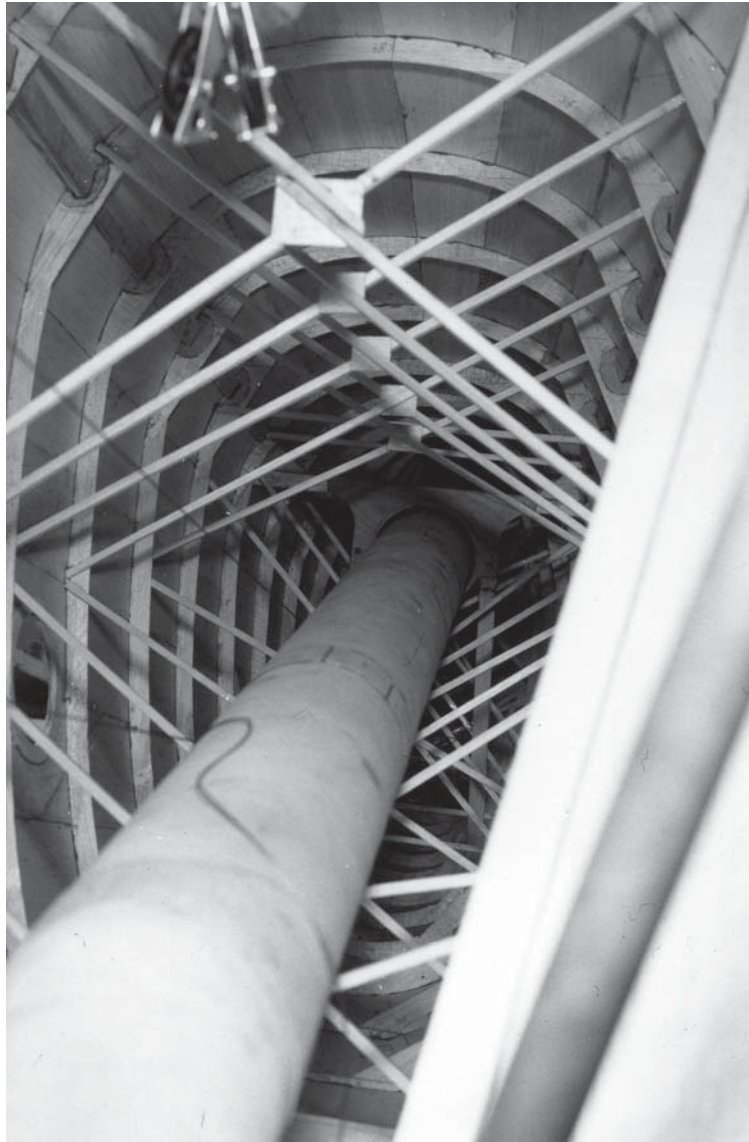
FIG 10. Laminated Balsa propeller drive shaft. 3 x 1/32" laminations of Balsa at +/- 45 degrees.
