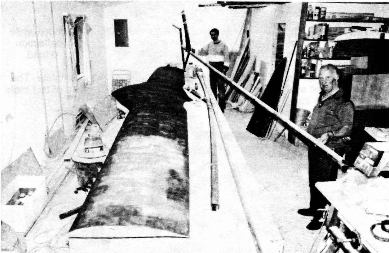
Figure 3. Showing the wing spar and wing centre section mould
