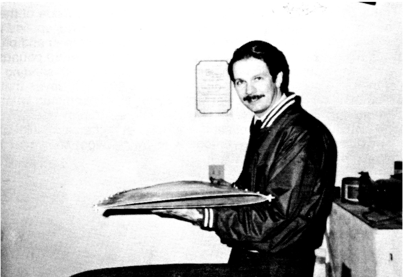
The mould construction techniques were similar for all the moulds. Figure 7 above shows the horizontal tail female mould. The alignment bolts used for part assembly can be seen on the mould flanges
