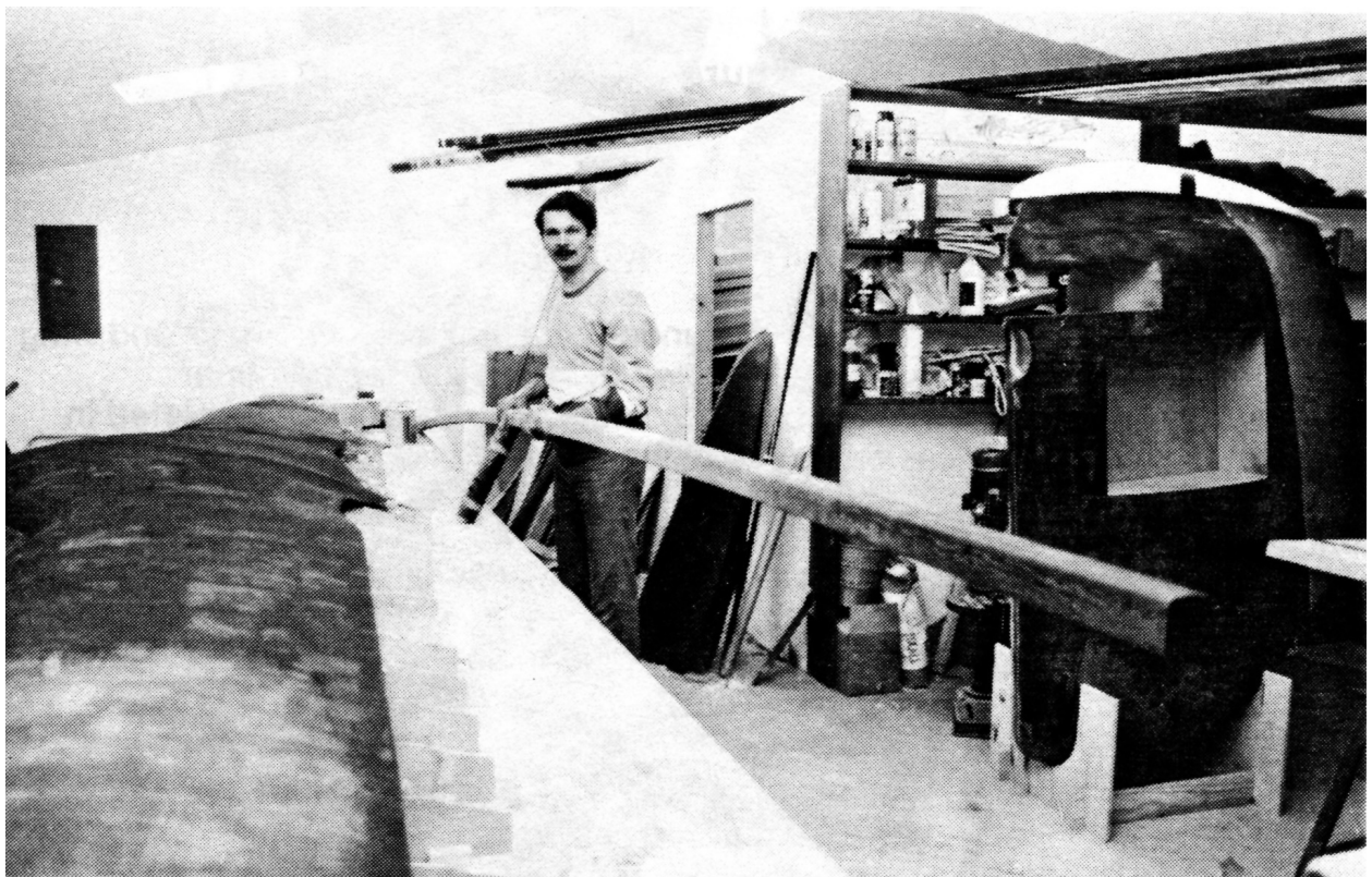
Figure 4. Showing the anhedral built into the centre spar. The fuselage mould is shown on the right
