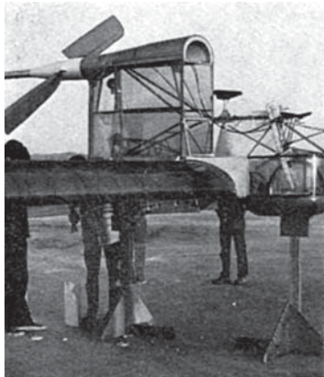
Like a microfilm indoor model on its stand, Icarus being assembled in El Mirage dry lake, California Prop stands are needed for wing assembly, with one person at each tip All fairings are from foam sheet. Photos by Joel Rieman.
