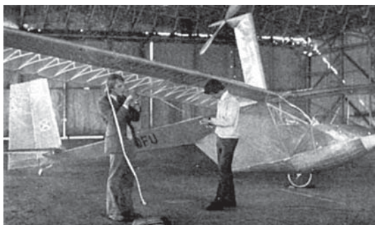
Like a microfilm indoor model on its stand, Icarus being assembled in El Mirage dry lake, California Prop stands are needed for wing assembly, with one person at each tip All fairings are from foam sheet. Photos by Joel Rieman.
