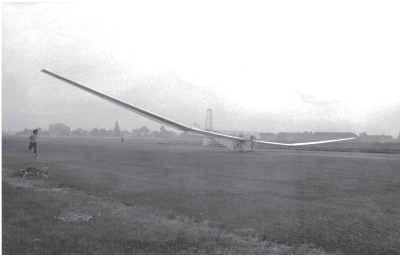
Figure 25. Banking while close to the ground can produce a heart stopping moment. Small outrigger wheels at the wing transport joints are provided to keep the outer wings off the ground in such an event.
