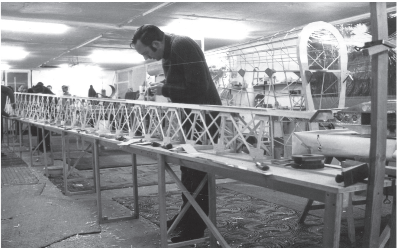
Figure 12. Outer wing torsion box. Before construction could begin the 50 ft. table had first to be levelled and firmly secured to the concrete floor. Due to the wing taper, every rib is different.
