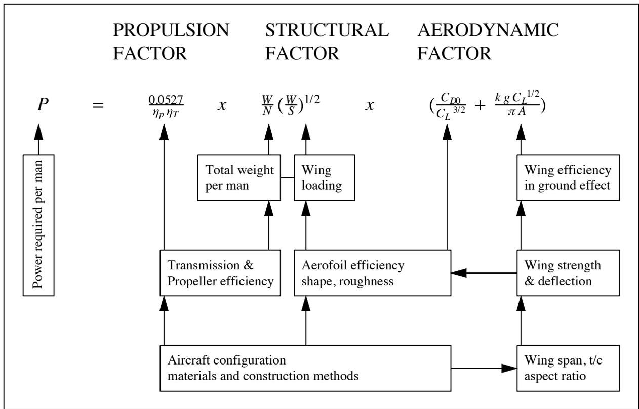
Fig 6: Structural Design Influence on Power Requirement
