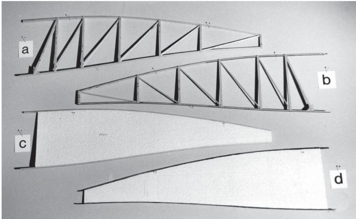
Experimental ribs suitable for a single seat aircraft. Total chord 1.5 m
