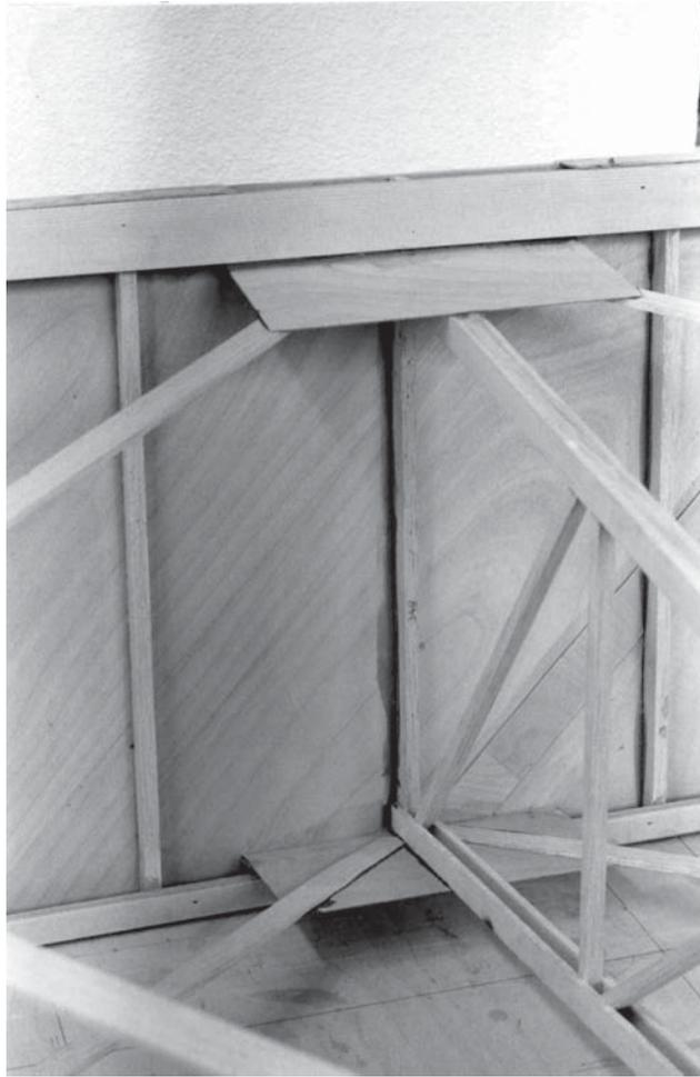
Twin flange main spar with diagonal web and capping, balsa stiffeners, main ribs and spruce diagonal bracing.
