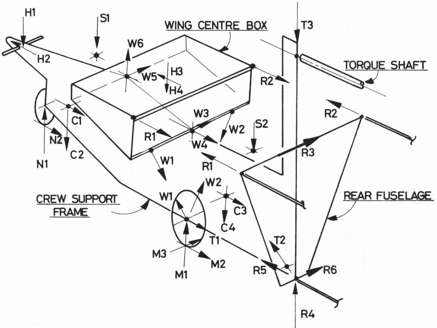
Fig 12: Major Forces Arising at the Wing Fuselage Intersection of Toucan 1
