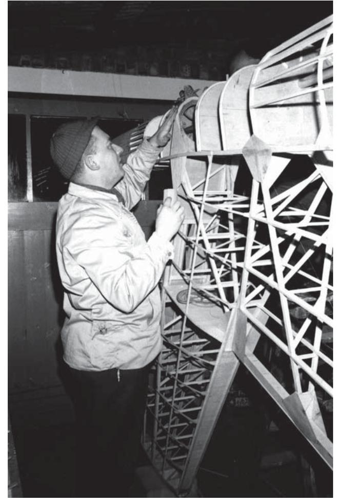
Martyn Pressnell working on the fin attachment frame and propeller shaft fairing, jugged on the shaft itself for alignment.
