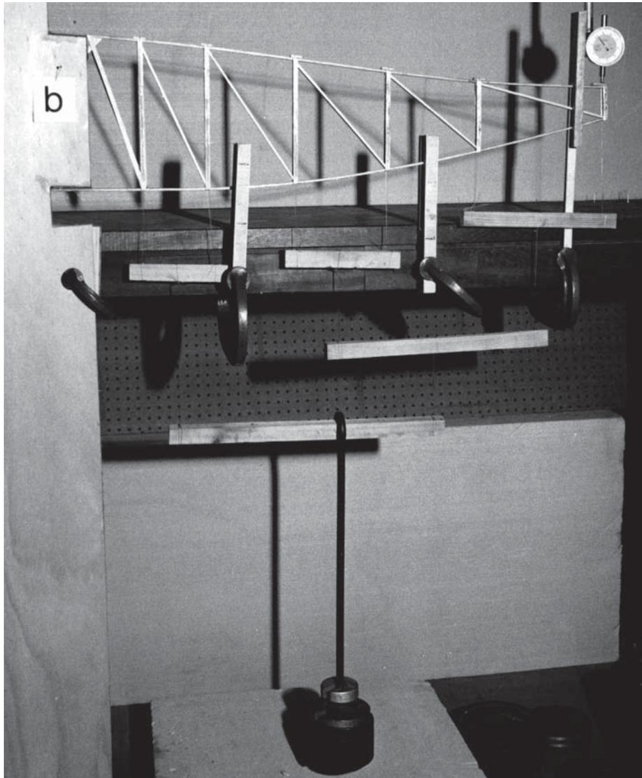
Method of loading the ribs in the test
