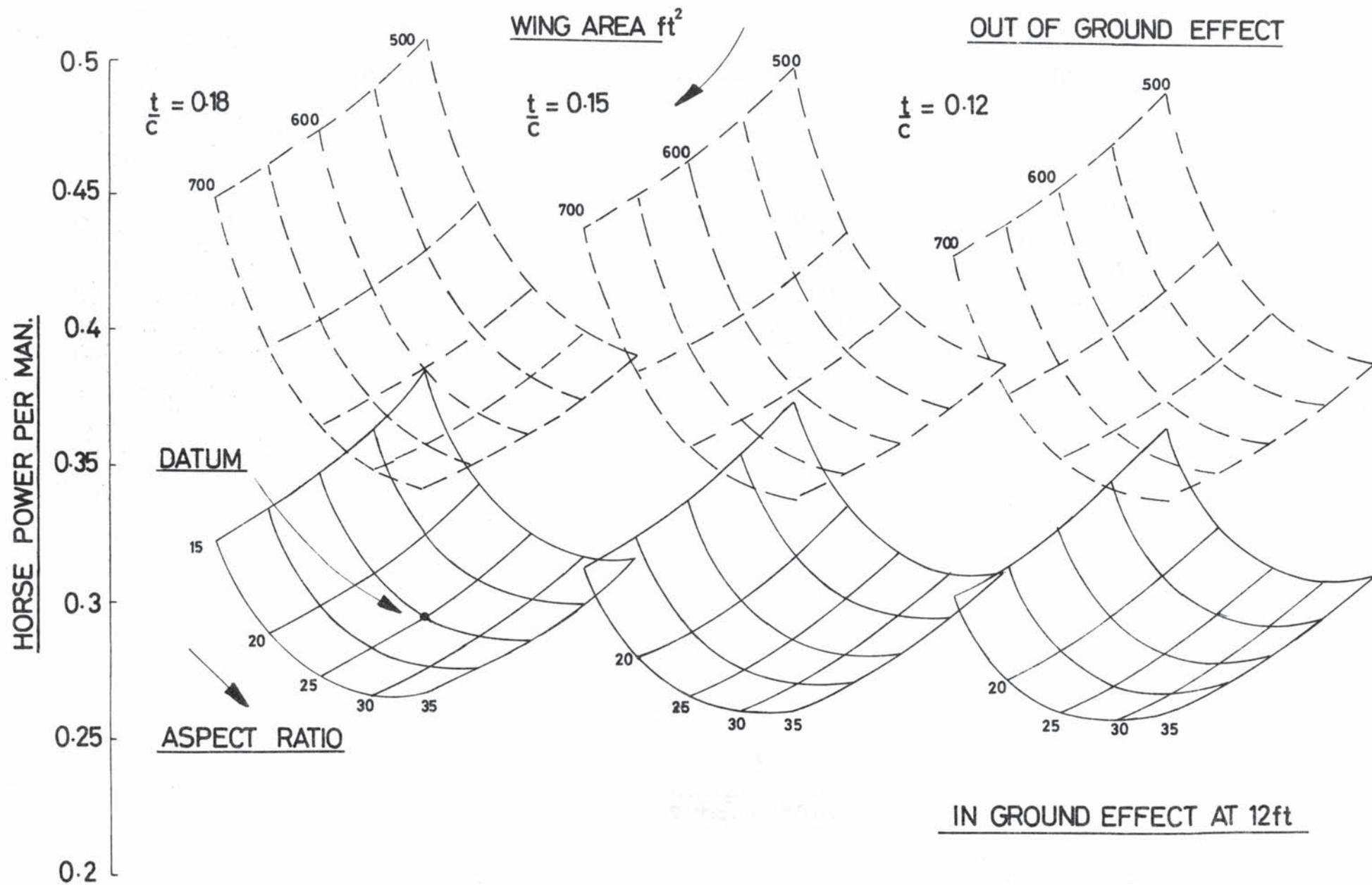
Fig 8: Two Seat Aircraft Power Requirement  $C_L = 1.0$
