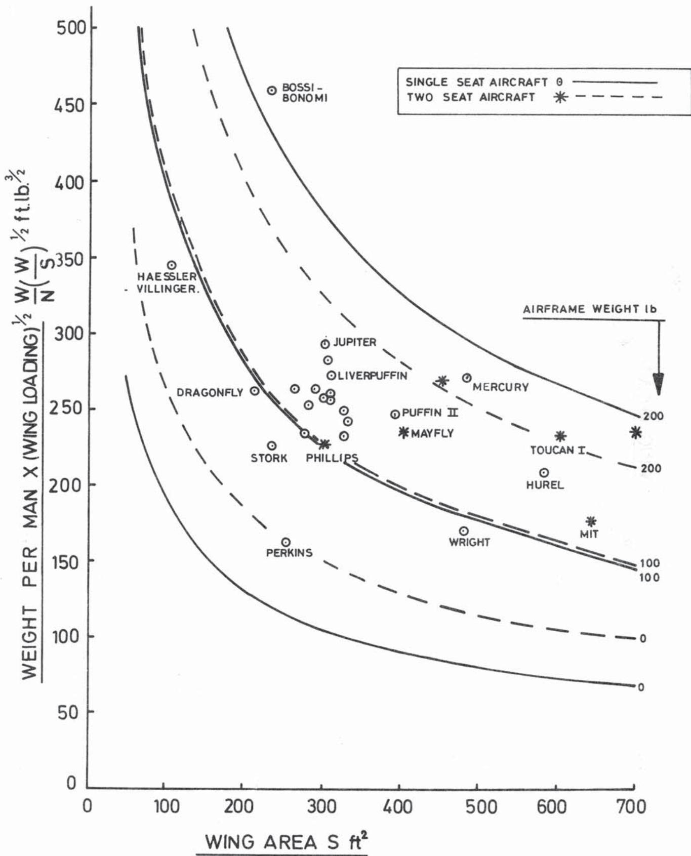
Fig 7: Man-Powered Aircraft Relative Performance Structural Factor
