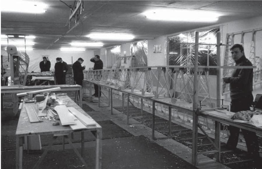
Wing assembly, spruce and ply spar, balsa nose spar and ribs
