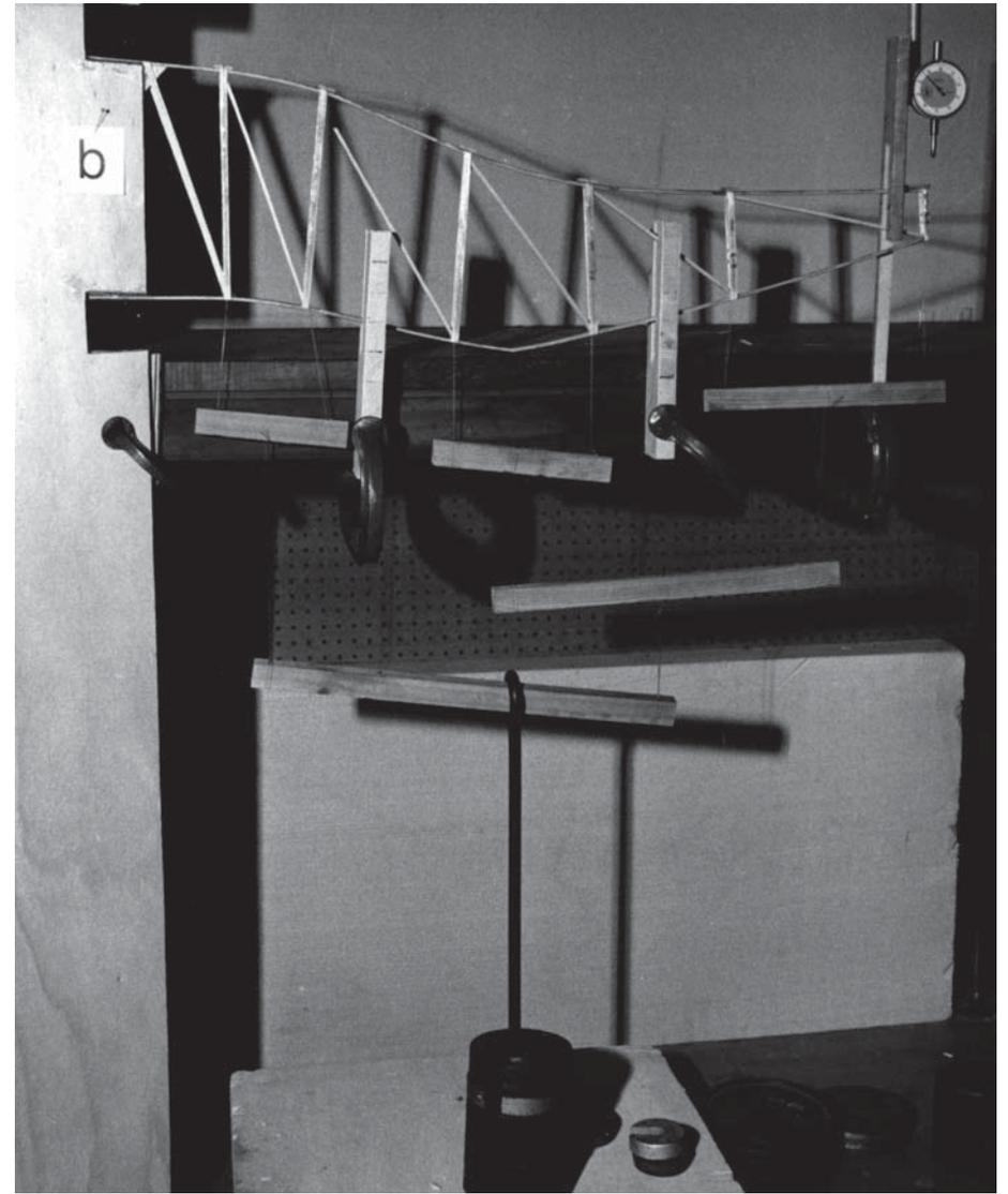
Rib (b) following failure of a joint in the shear bracing
