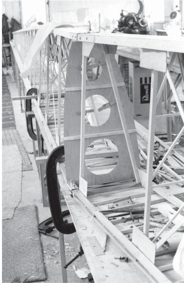
Inner wing main box stub at transport joint, alignment for dihedral. Tapering aluminum lug reinforcements, flange and shear links.
