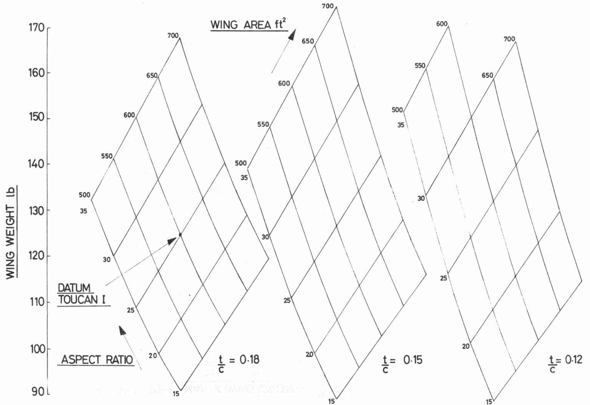
Fig 8: Two Seat Aircraft Wing Weight
