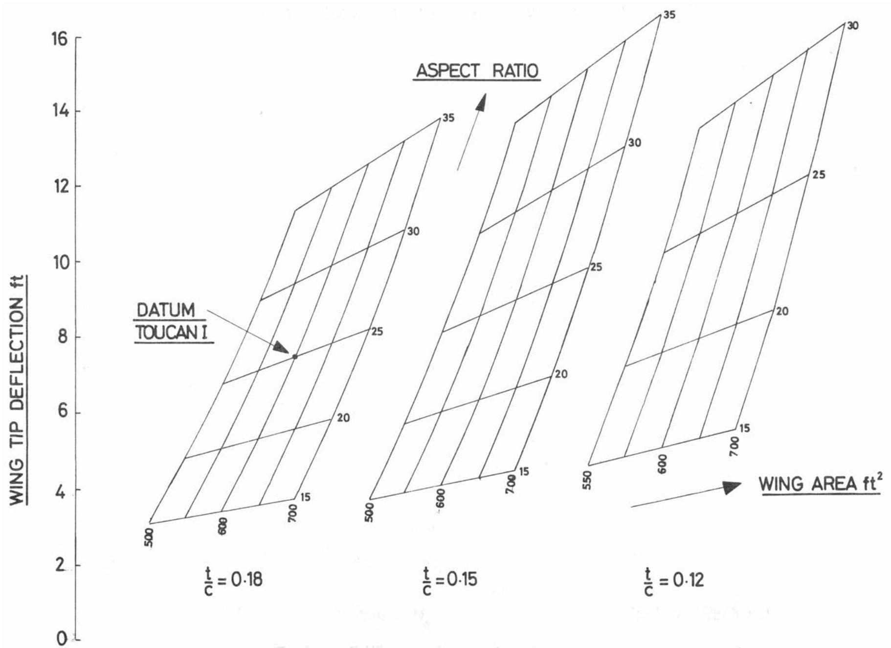
Fig 9: Two Seat Aircraft Wing Tip Deflection
