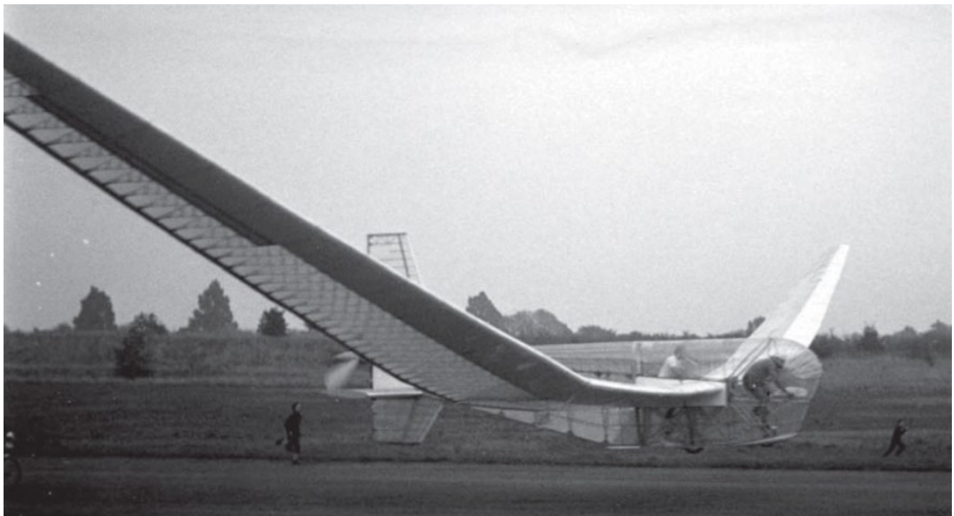
TOUCAN I airborne at Radlett Airfield where its best flight covered a distance of 700 yards (640 m) in July 1973. It is the only two-seat aeroplane to have flown to date, and the modified aircraft TOUCAN II is the largest machine to be constructed, with a wingspan of 139 ft (42.37 m).
