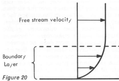
Considering flow over an aerofoil section the boundary layer starts from the front and builds up in thickness as the flow travels along the section. The boundary layer over the front of the section will be laminar but as the thickness increases the flow becomes unstable and transition takes place to a turbulent boundary layer. For low skin friction drag it is important for the laminar boundary layer to remain stable over
