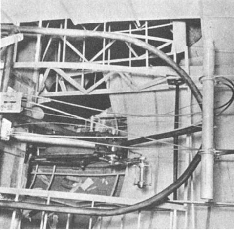
Looking down into Linnet III cockpit the cycling position, control bar, metal tube frame and cable controls are evident.
