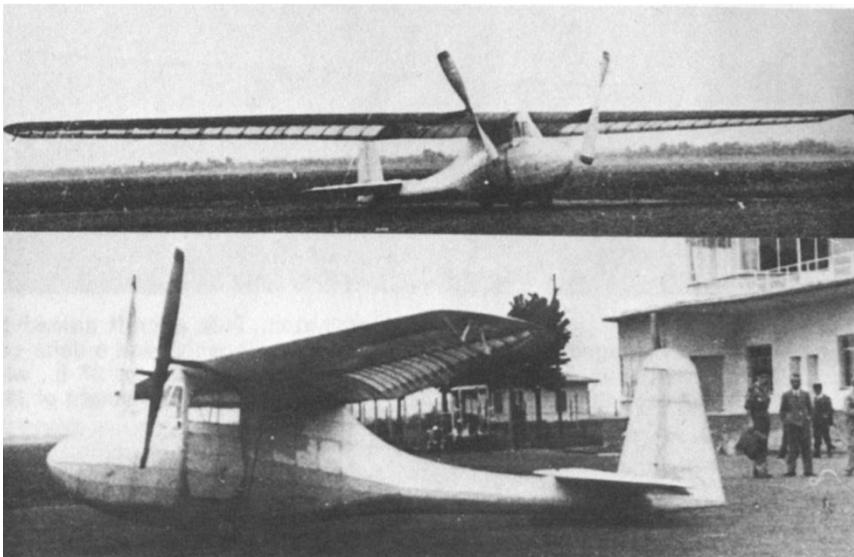
*Two views of the Bossi-Bonomi aircraft illustrate the contra-rotating propellers and the pronounced undercamber of the low speed aerofoil.*
