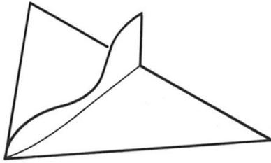
To ascertain whether the delta configuration has any practical possibilities for man-powered aircraft let us consider the simple configuration shown in Figure 75. With a wing span of 35 ft and a total length of  $17\frac{1}{2}$  ft, the wing area would be 306 sq.ft. Aspect Ratio =  $\frac{35}{8.75} = 4$
