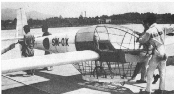
Above: the Japanese Nakamura MP-X-6 which is very much a one-man project, using the twin boom layout with pusher propeller at the rear of the pilot's nacelle. Underneath, the more successful Sato-Maeda SM-OX which has flown on many occasions in Japan.
