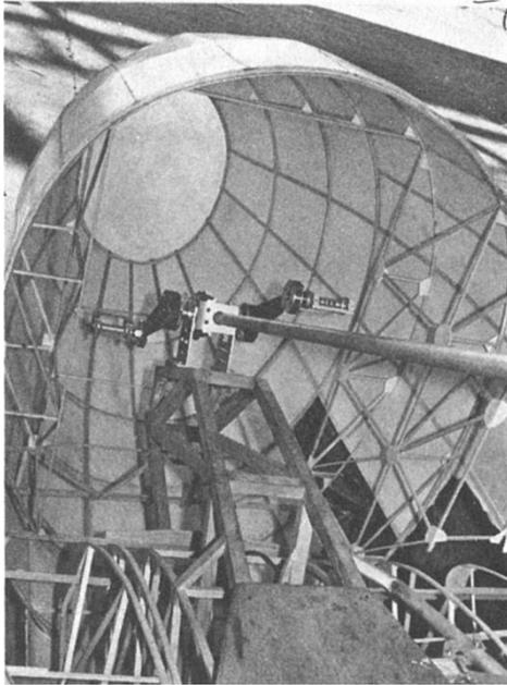
Below: on Linnet I, the prop shaft from the pedal driven bevel gears in the nose inclined up and rearwards to a horizontal shaft with universal joint, ball race supported and subsequently covered by large bullet fairing.
