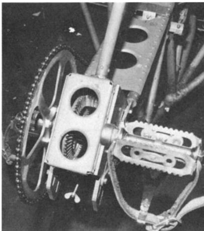
*Bevel gear transmission and chain drive for road wheel on the Weybridge machine.*
