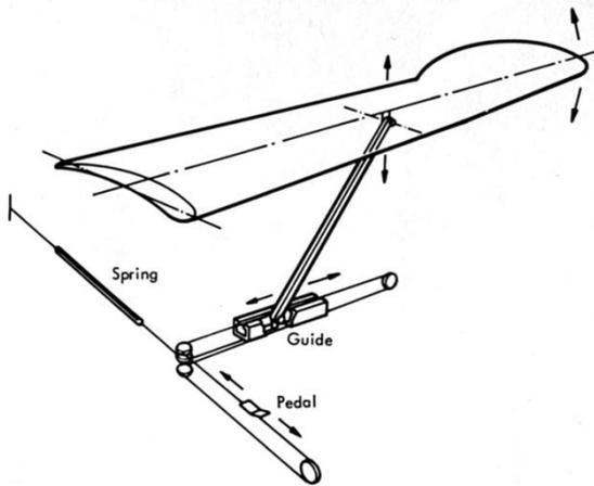
Figure 2 Operating mechanism of the Lippisch aircraft
