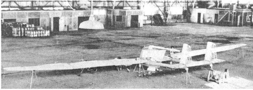
Above, assembly of the Nakamura man-powered machine in a Tokyo hangar in 1969 reveals the short twin boom fuselage (19 ft 8 in overall length) and the high aspect ratio of the 69 ft wings. Area is 226 sq ft and the aerofoil section is Gottingen 532; see below for transport joints including area where propulsion nacelle fits on to wing centre section.
