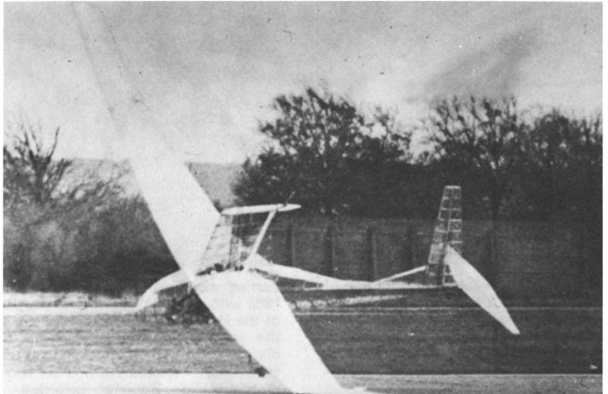
*Moment of disaster, SUMPAC crumples its wing and sustains other damage after stalling from 30ft. It is preserved in a repaired state at the Shuttleworth Collection, Old Warden, Biggleswade, Bedfordshire<sup>5</sup>, as below.*
