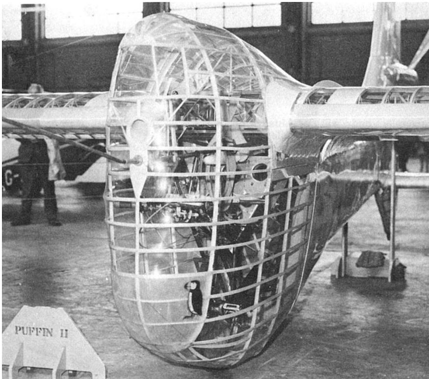
*Prior to its ultimate crash in collision with airfield equipment, Puffin II had been developed up to a state of aerodynamic cleanliness few other Man-Powered aircraft could hope to match. Note the symbol on the front cowling, and the wing fairings.*
