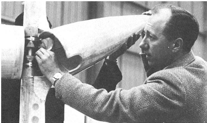
*The Spinner on the Puffin prop hub is retained by rubber bands and removes easily for access to the blade clamps for any adjustment of propeller pitch. Note the added cuffs at the blade root.*
