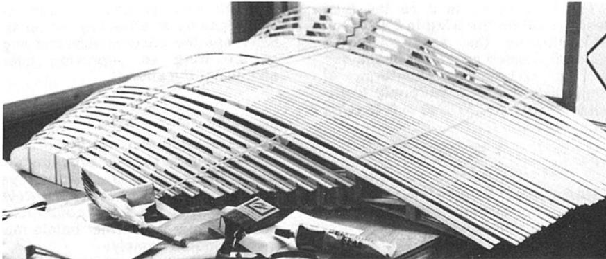
Positioning of the spar in the wing must be such that twisting of the wing is minimised under aerodynamic loading. Generally the pressure on an aerofoil tends to act about a centre of pressure at approximately  $\frac{1}{3}$ <sup>rd</sup> chord back from the leading edge and to minimise twisting of the wing this is the point at which to place the spar. Figure 65 shows the box spar in position in the Wortmann FX-63137 section.
