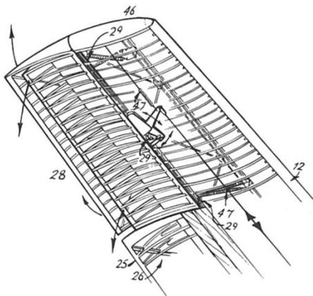
**12.** Sorboprene leading edge covering. **25.** 3/32 in Balsa trailing edge. **26.** Normal ailerons. **28.** Drag rudders. **29.** Hinges. **46.** Balsa tip. **47.** Return spring.
