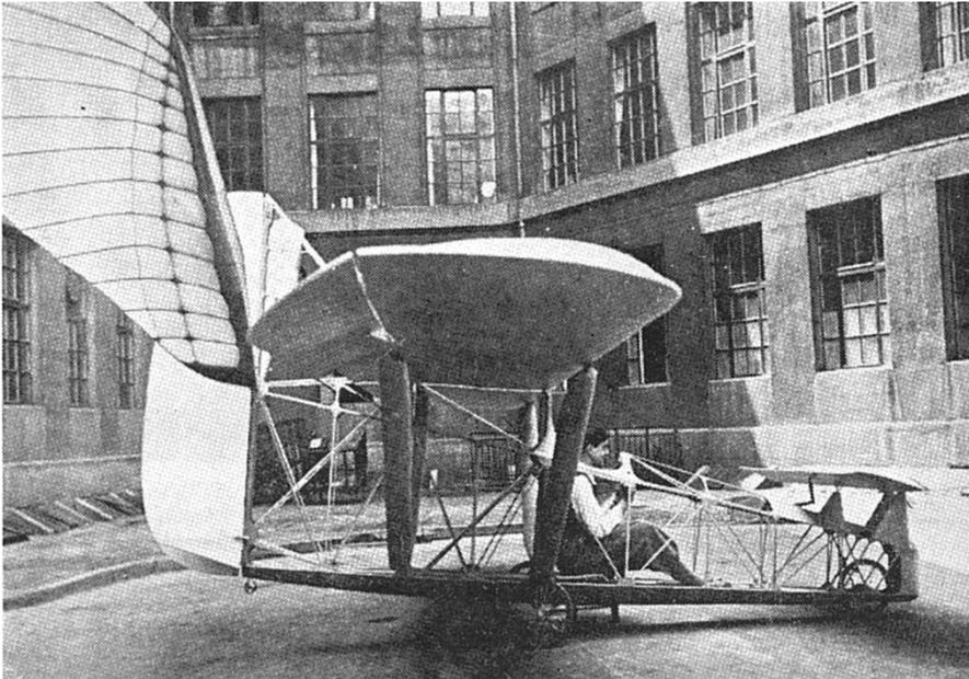
Full sized and model ornithopters have attempted to copy the insect motion since it represents the simplest flapping mode. Success has been limited because the insect wing behaviour relies on very high frequency flapping which is impractical with larger devices.
