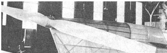
Left, the rigid, high aspect ratio propeller made by Eiji Nakamura. Below, the Weybridge aircraft propeller, and the adjustable pitch propeller of Puffin I and II, with lightening holes in balsa blades.
