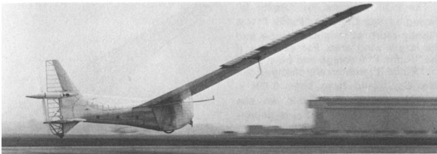
*The wing to fuselage fairings and side profile of the nose were changes in the Puffin II, seen above; with the Puffin MK I airborne at Hatfield.*
