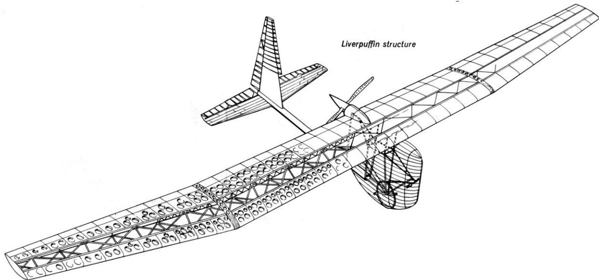
There could be no greater contrast than in the rear fuselage sections of the single seat liverpuffin (above) and the two seat Toucan (below).
