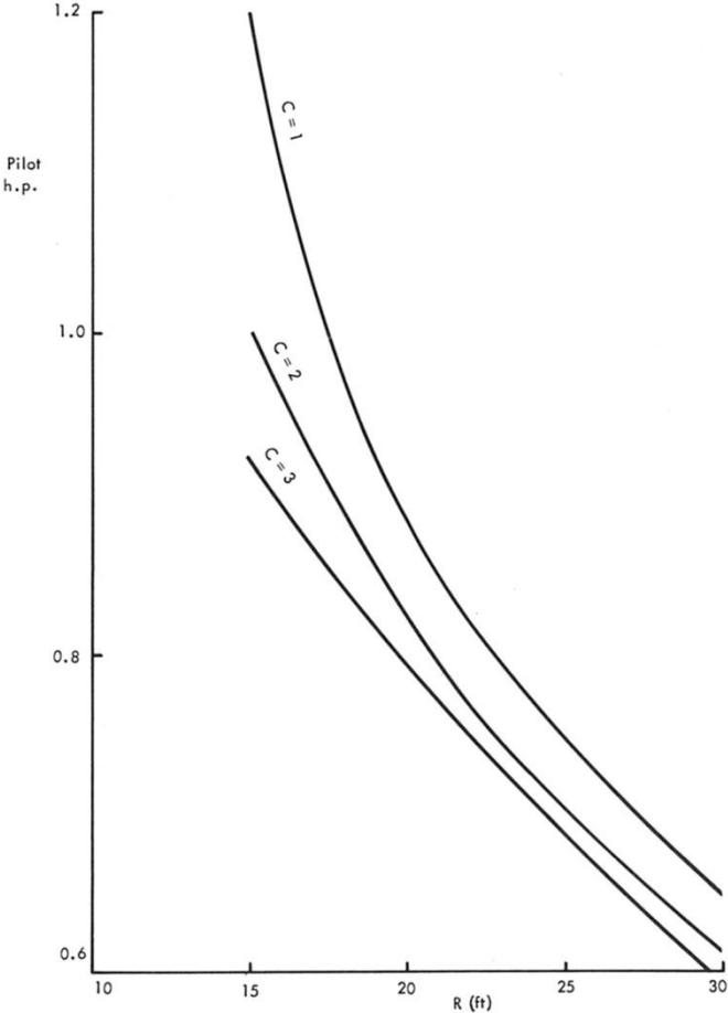
Figure 80 Variation of power with helicopter rotor radius
