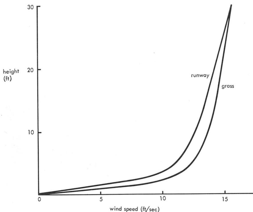
Figure 86 Variation of wind speed near the ground
