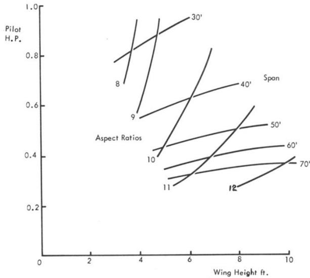
Figure 40 Power requirements for non-powered aircraft
