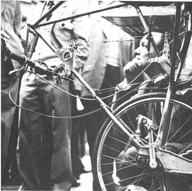
*Right: The road wheel and forward frame of Puffin II with the cable operated controls from the horizontal bar suspended at the forefront of the fuselage. Below right is the Puffin I tail unit showing the original horn balance for the comparatively narrow chord elevators. The balance was not used on Puffin II.*
