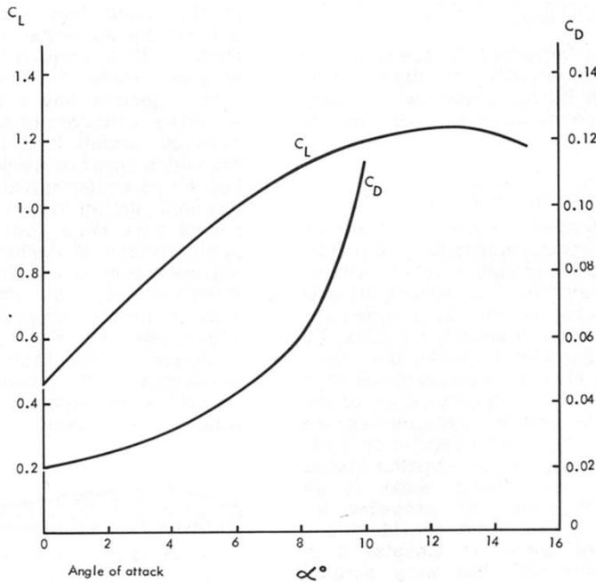
Figure 48 Performance curves for the 9% Clark Y aerofoil section
