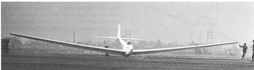
Take off by Linnet III showing the increased dihedral, inverted section tail at negative position and wing tip assistants holding skids.
