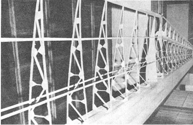
Top: collection of wing ribs, and at left, the assembled wing of the Nakamura man-powered aircraft illustrate use of a Leading Edge box spar arrangement.
