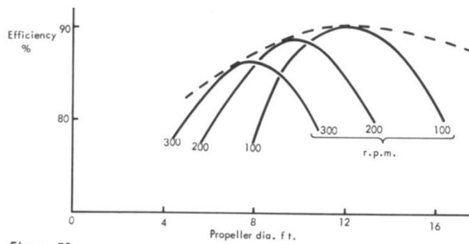
Figure 56 Variation of efficiency with propeller diameter
