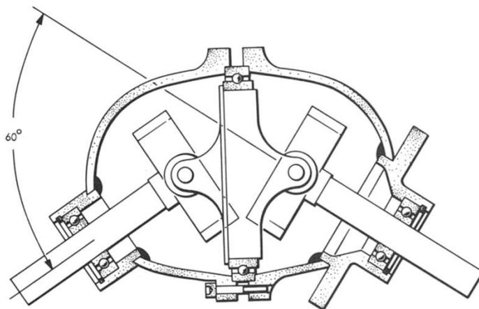
*Figure 42* Proposed gearbox design for a propeller drive mechanism.
