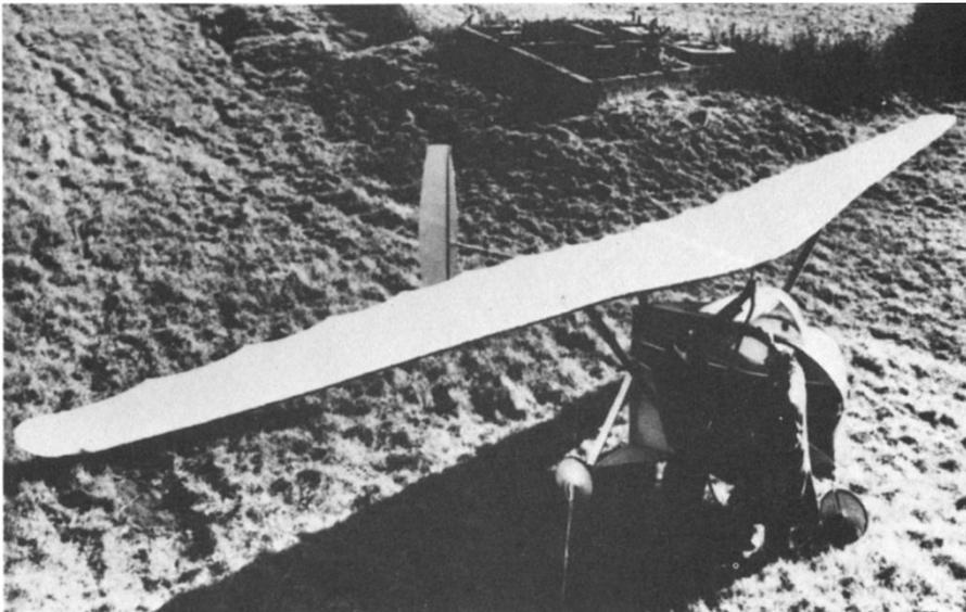
*First of four pneumatic airframes made by D. Perkins at Cardington was this tailless project made in the late fifties. It was not successful.*
