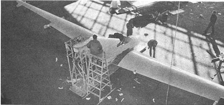
*Linnet Mk. 1 being assembled in a hangar by students of Nihon University Tokyo. The short moment arm of the rear fuselage and high aspect ratio of the wings are evident as well as the requirement for precise assembly jigs to cope with the size of structure.*
