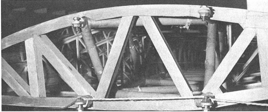
*Combination of metal tube wing spars and balsa ribs for the Weybridge machine is in part influenced by use of articulated wing panels for lateral control. This is a semi span transport break joint.*
