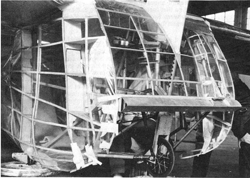
*Side by side seating in the reclining position was chosen for the Southend two-man machine resulting in a blunt, broad nose.*
