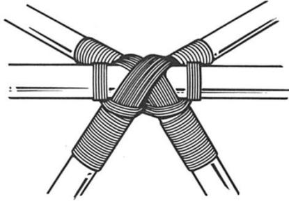
Laced joint for thin metal tubes.
