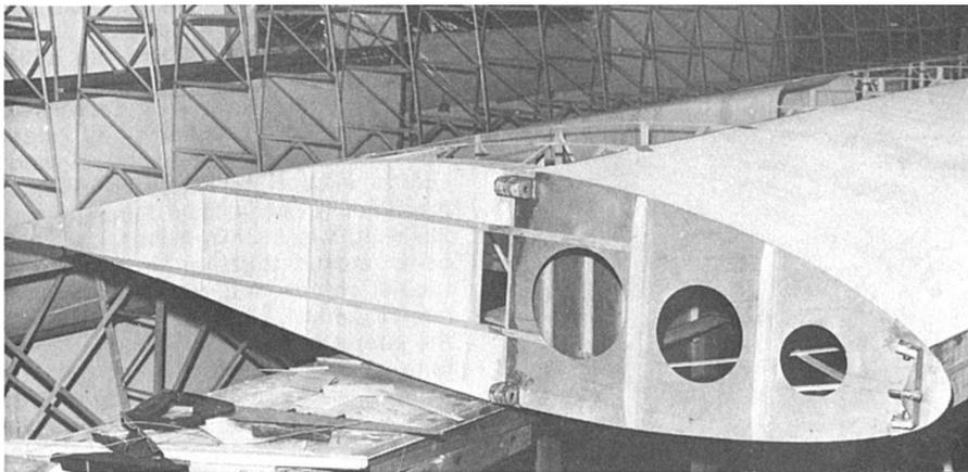
*Transport break at semi-span on Toucan has provision for the dihedral adjustment about the chord line indicated by the pickup at the leading edge here, and with variable links at the two spar joint lugs on the plywood and sheet balsa faced end rib.*
