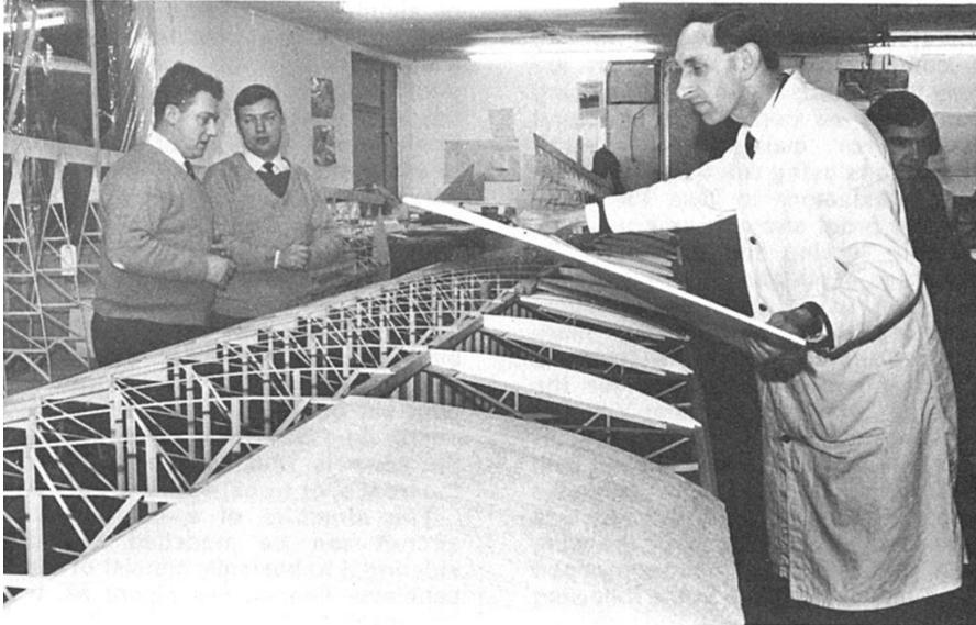
*Leading edge section of Toucan is sheathed in expanded polystyrene supported by sub ribs of the same material. Application, and results of test sections have proved extremely successful.*
