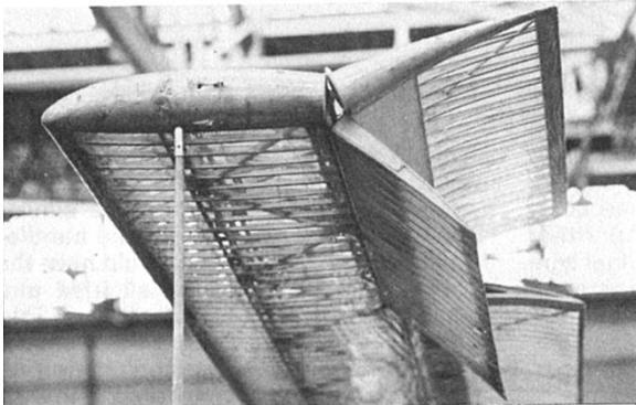
*The Puffin II drag rudder used at the wing tips to improve control. At first this was coupled with rudder but was later disconnected. Above the panels are in the open position. below, closed, also revealing close rib spacing.*
