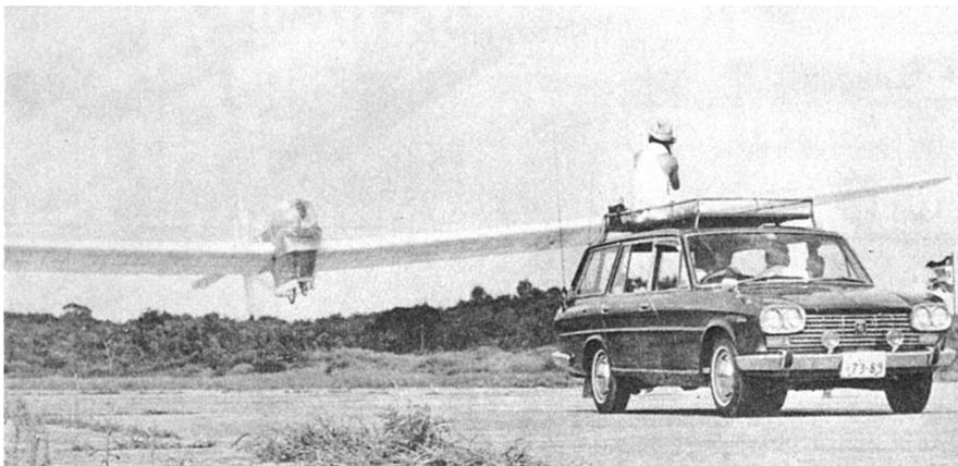
First assembly of the Maeda SM-OX shows the constant chord centre panel and tapered tips of this machine designed by a 22 year old.
