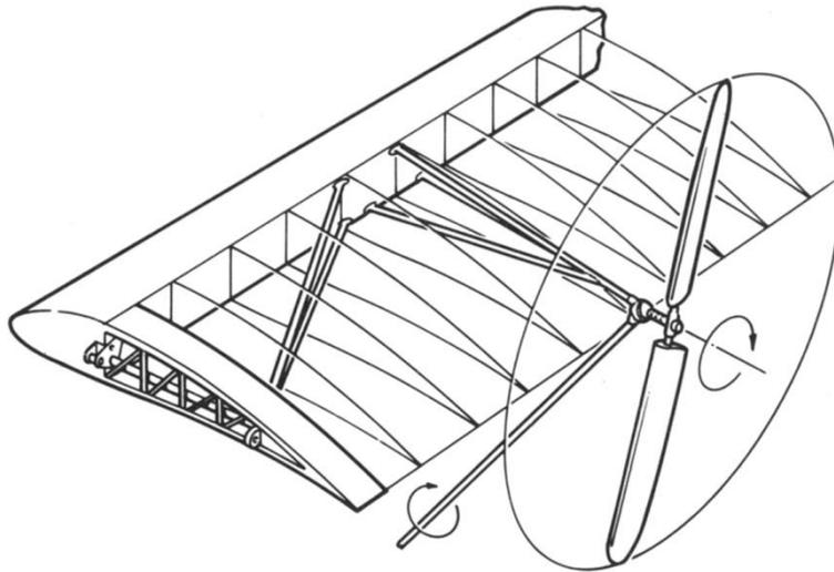
Propeller arrangement Ottawa aircraft
