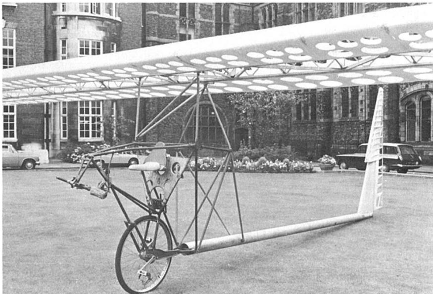
*Posed in the august surroundings of Liverpool University, Liverpoolpuffin basic structure with rear fuselage boom is seen here. A belt and shaft drive is used to drive the propeller and the road wheel.*
