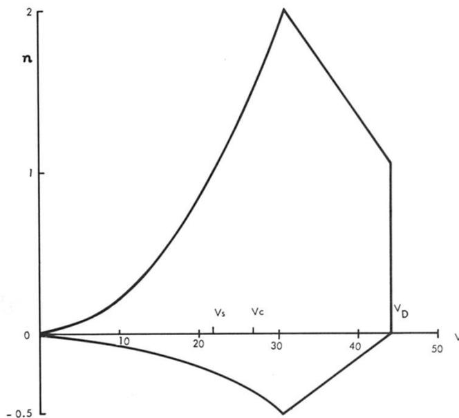
Figure 60 Typical non-powered aircraft manoeuvring envelope
