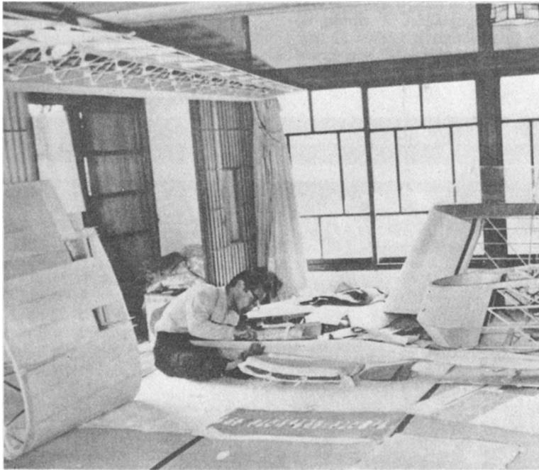
*Eiji Nakamura working single handed on his 69 ft span MP-X-6 machine prior to completion in 1969. Airframe weight was 132 lbs. First tests were unsuccessful due to structural failure.*
