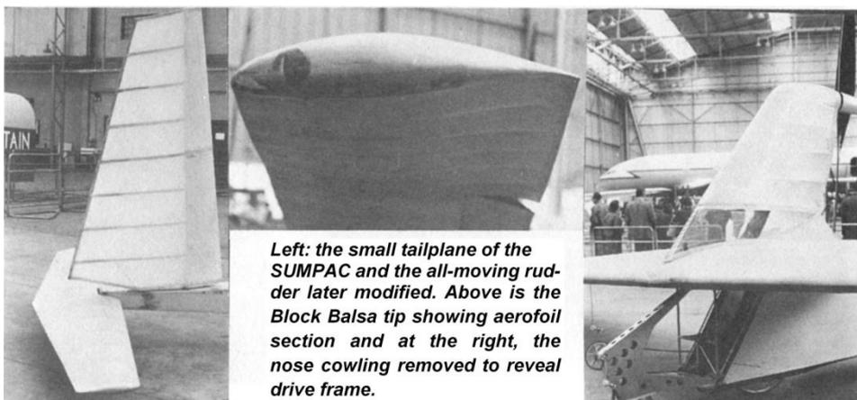
Left: the small tailplane of the SUMPAC and the all-moving rudder later modified. Above is the Block Balsa tip showing aerofoil section and at the right, the nose cowling removed to reveal drive frame.
