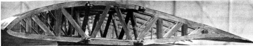
*Above: the Weybridge wing at semi-span joint, the entire surface can be rotated for lateral control.*
