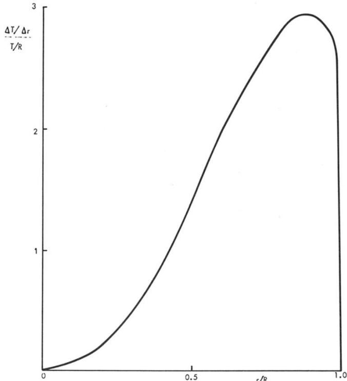
Figure 55 Generalised thrust grading variation with propeller radius
