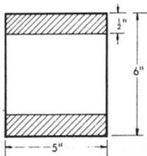
Would this spar be suitable if the top and bottom flanges are constructed of spruce?
