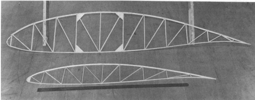
*Experimental rib structures for the Weybridge aircraft utilising Tee section booms and braces.*
