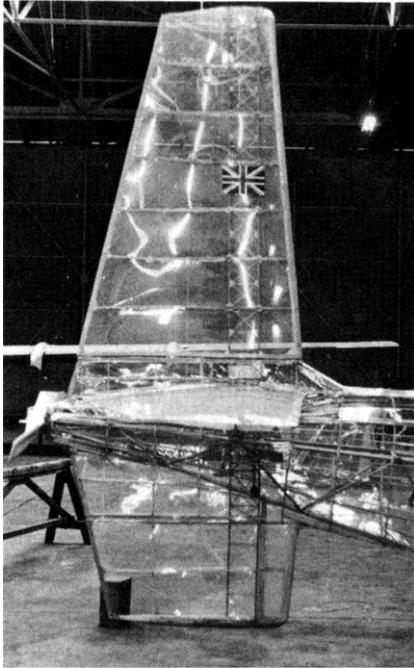
*Of all the Man-Powered aircraft projects the Weybridge machine control system is the most adventurous. All the surfaces are moveable except for the small fixed area at top and front of lower fin (above).*
