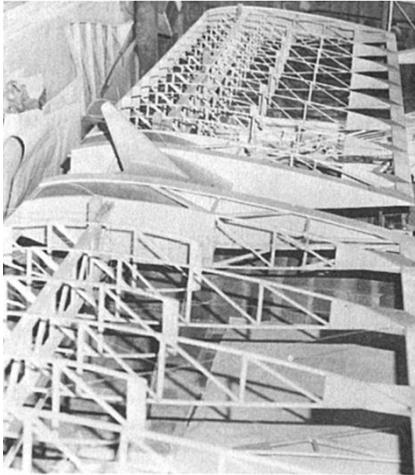
*The one piece all-moving elevator of Toucan (above) is actuated via the projecting horn through a cam control (below) giving a positive trim rather than proportional feedback. to the control-column.*
