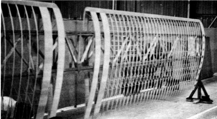
*Above, the close rib spacing of the revised centre section on Puffin II, seen prior to assembly on the fuselage. Below, a profile of the Puffin II tail showing the enlarged rudder, and removal of horn balance on the elevators.*
