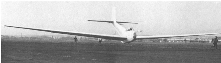
Take off by Linnet II in 1967. Pilot position had been changed from that of Linnet I. Tailplane is modified to an inverted section at this stage.
