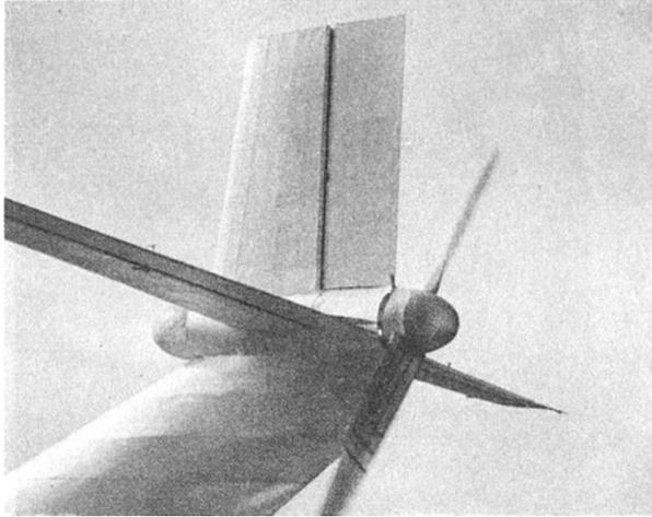
*Above, the acorn fairing on Linnet I filled after first flights to streamline the layshaft arrangement which picked up drive from the pilot's pedals and shaft via bevels.*
