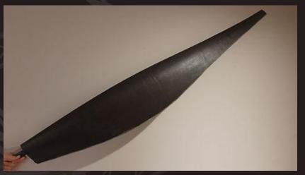
More recently, Charles D'Henin of Lazarus has had success with hollow printed cores and monocoque carbon outer layers
