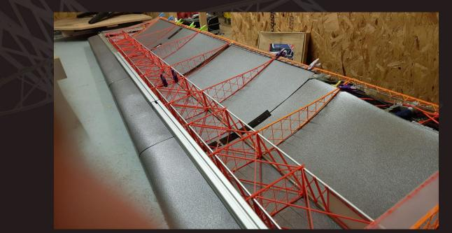
Start with box section spar - two identical trusses with carbon tube caps:
