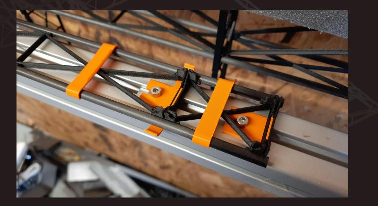
Slot center ribs into the truss tabs, followed by the second truss:
