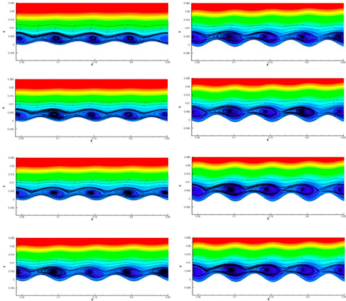
Structure of airflow over water waves, showing smoother air flow as altitude increases. Remember that though the wind may be light there may also be a less visible long wave swell running that the wind must flow over.
