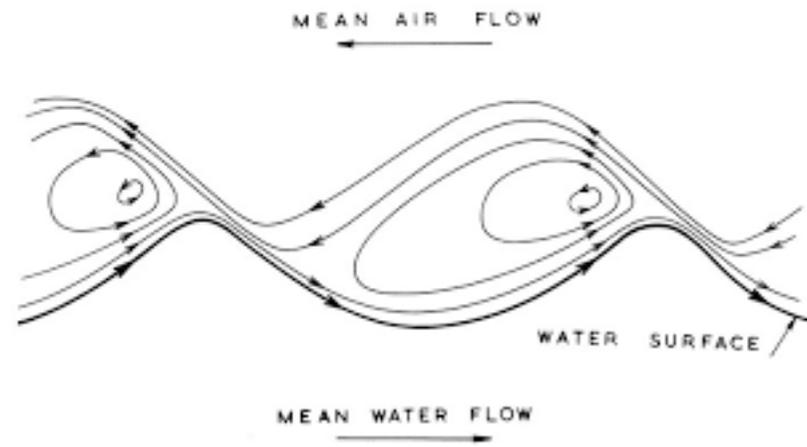
Structure of airflow over water waves.
