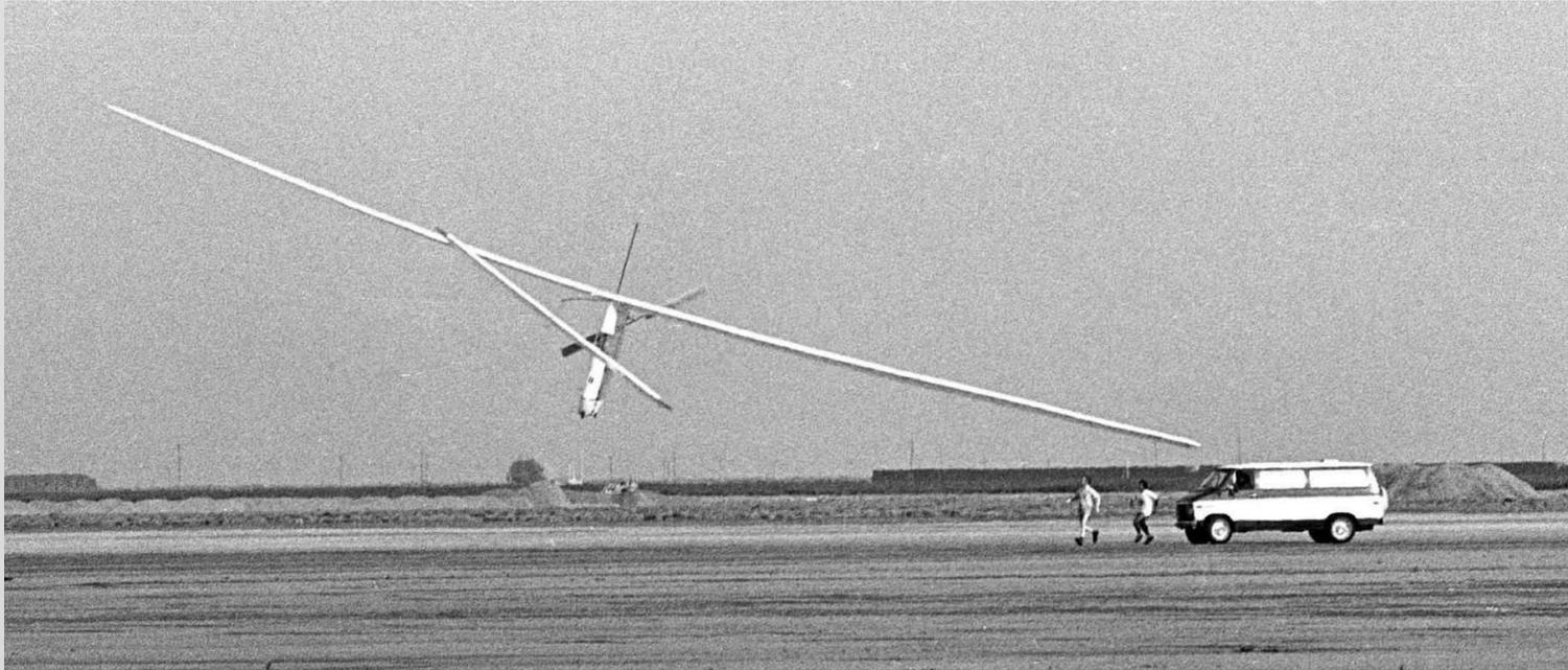
Loss of control, 1978 @ Shafter. due to control-system failure; I still have scars. Substantial structural damage from this and *five* other crashes, plus modifications made for transportability, led to this craft (GA #1) gaining **fifteen pounds** from its original fifty-five pounds
