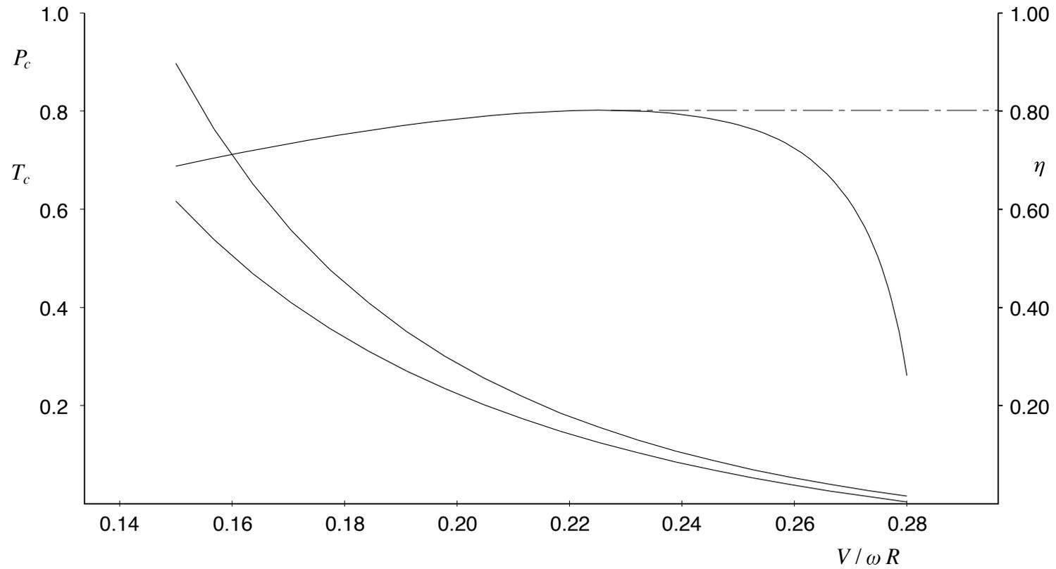
Calculation of Gossamer Condors propeller efficiency, using the drawings from Paul MacCready's plans set and XROTOR
