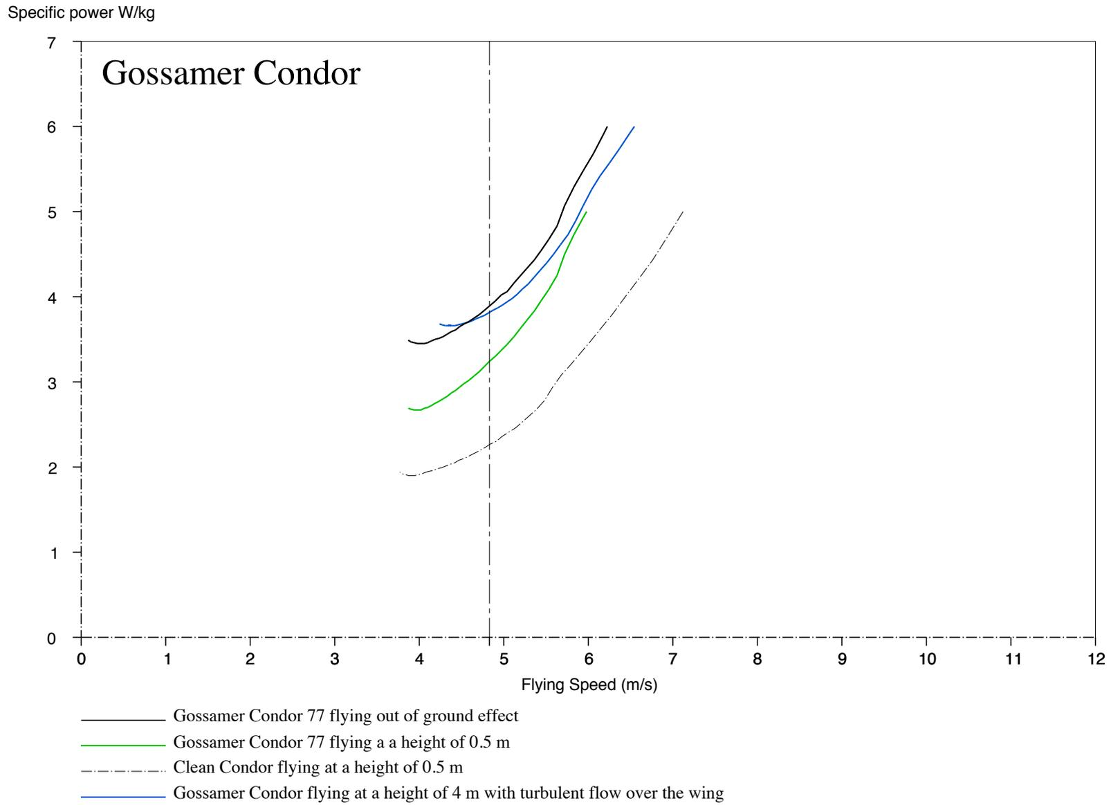
Figure 1. Calculated power polars for Gossamer Condor for several assumptions.
