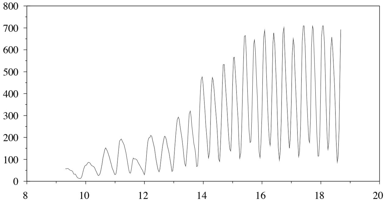
Fig. 10. Power during take off from the power meter. The raw signal is integrated to obtain the average power needed to fly.
