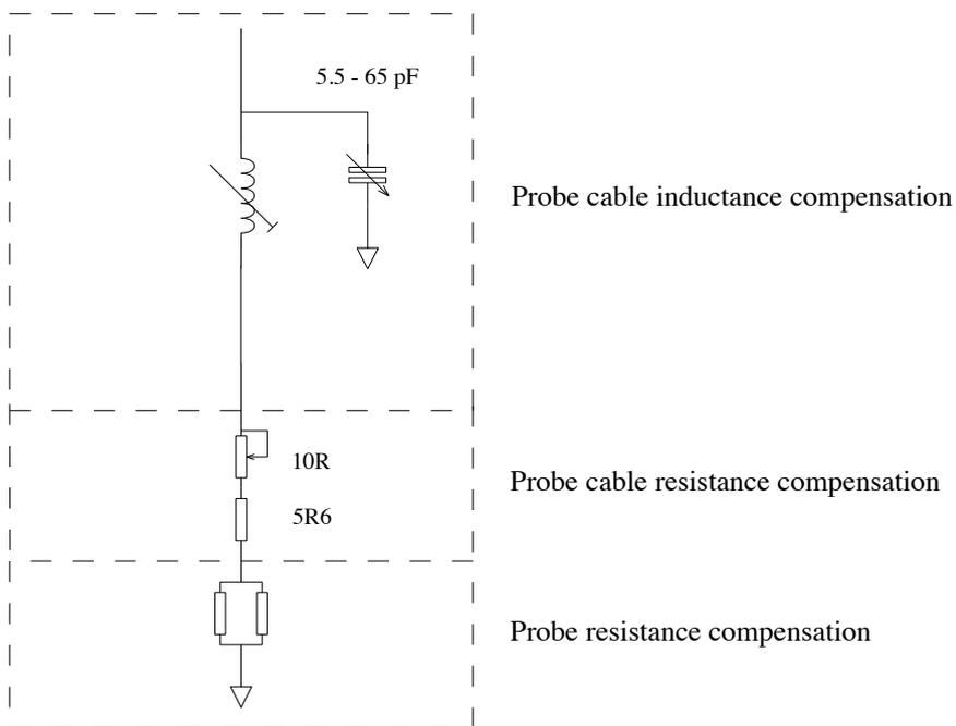
The variable inductor is made from 60 turns of insulated copper wire wound onto RS coil formers 228-090
