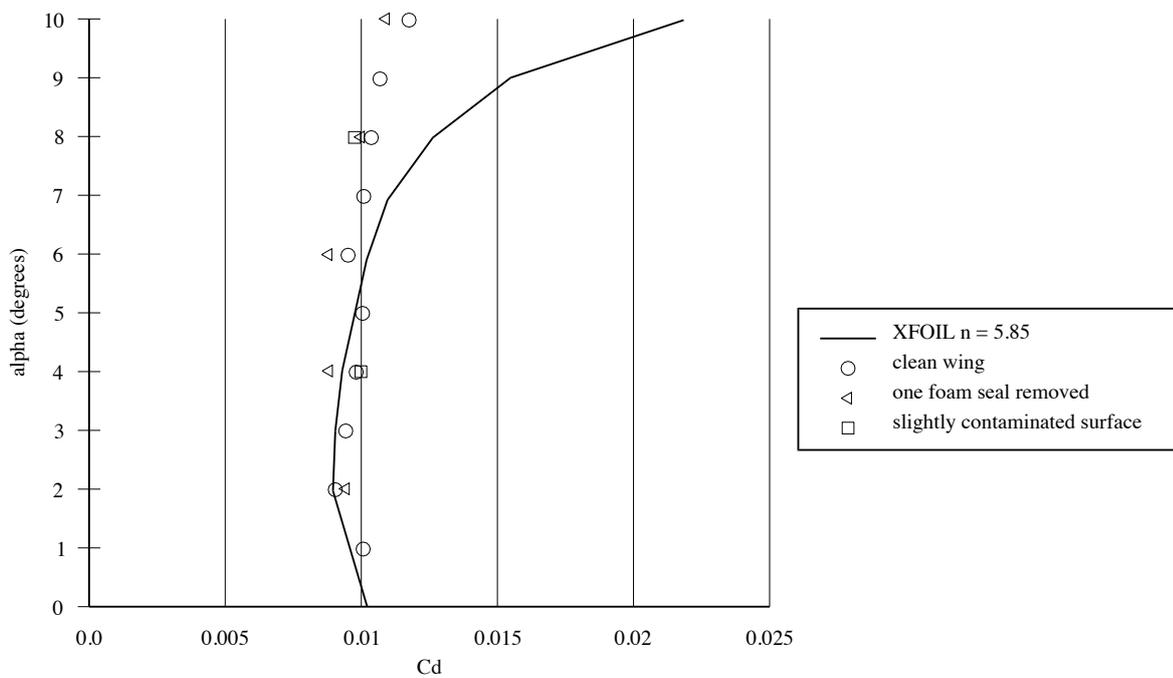
Fig 9.2 Theoretical and experimental drag values for rms free stream turb. Intensity = 0.26%
