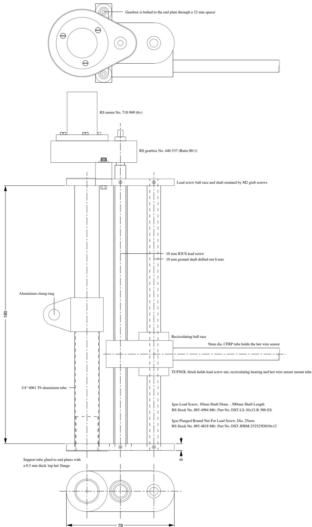
Appendix B. Drawing of the wake traverse used to measure drag in a wind tunnel and in flight. This drawing was drawn full sized and scaled to fit here. A few dimensions are given for anyone wishing to copy it. Note. Many CAD programs will import pdf format so it is easy to import this drawing and scale it back up to full size.
