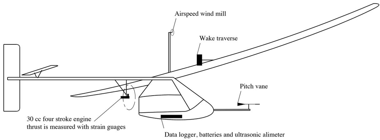
Figure 1. Airglow HPA instrumentation
