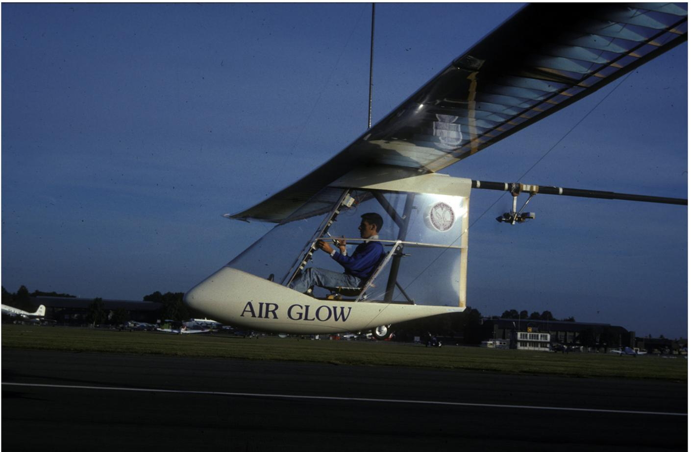
Figure 3. Airglow HPA flying with a small i.c. engine mounted using a strain gauged strut to measure thrust in flight.
