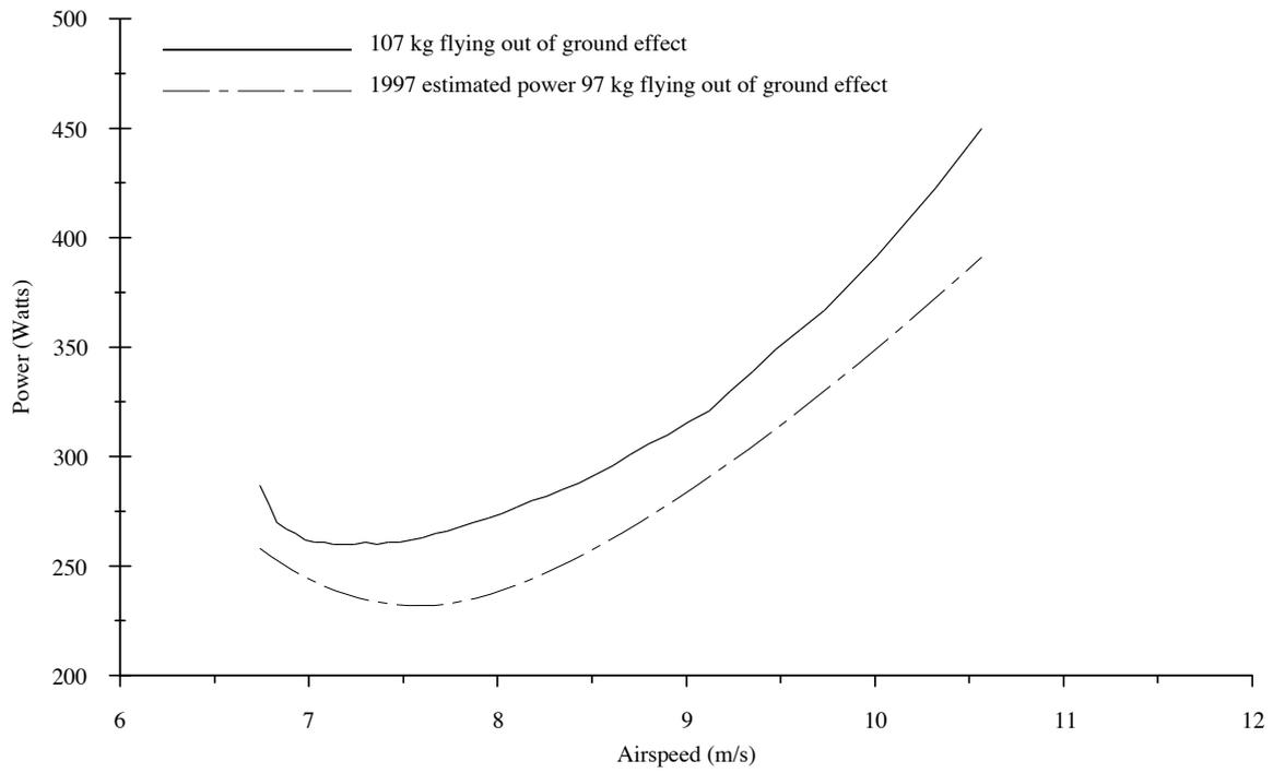
Fig. 12. Power polar calculated in 1995 using a lifting line model and plausible estimates (I now suspect they were under estimates) and a power polar calculated using a 3d panel code and more detailed estimates for individual components drag etc.
