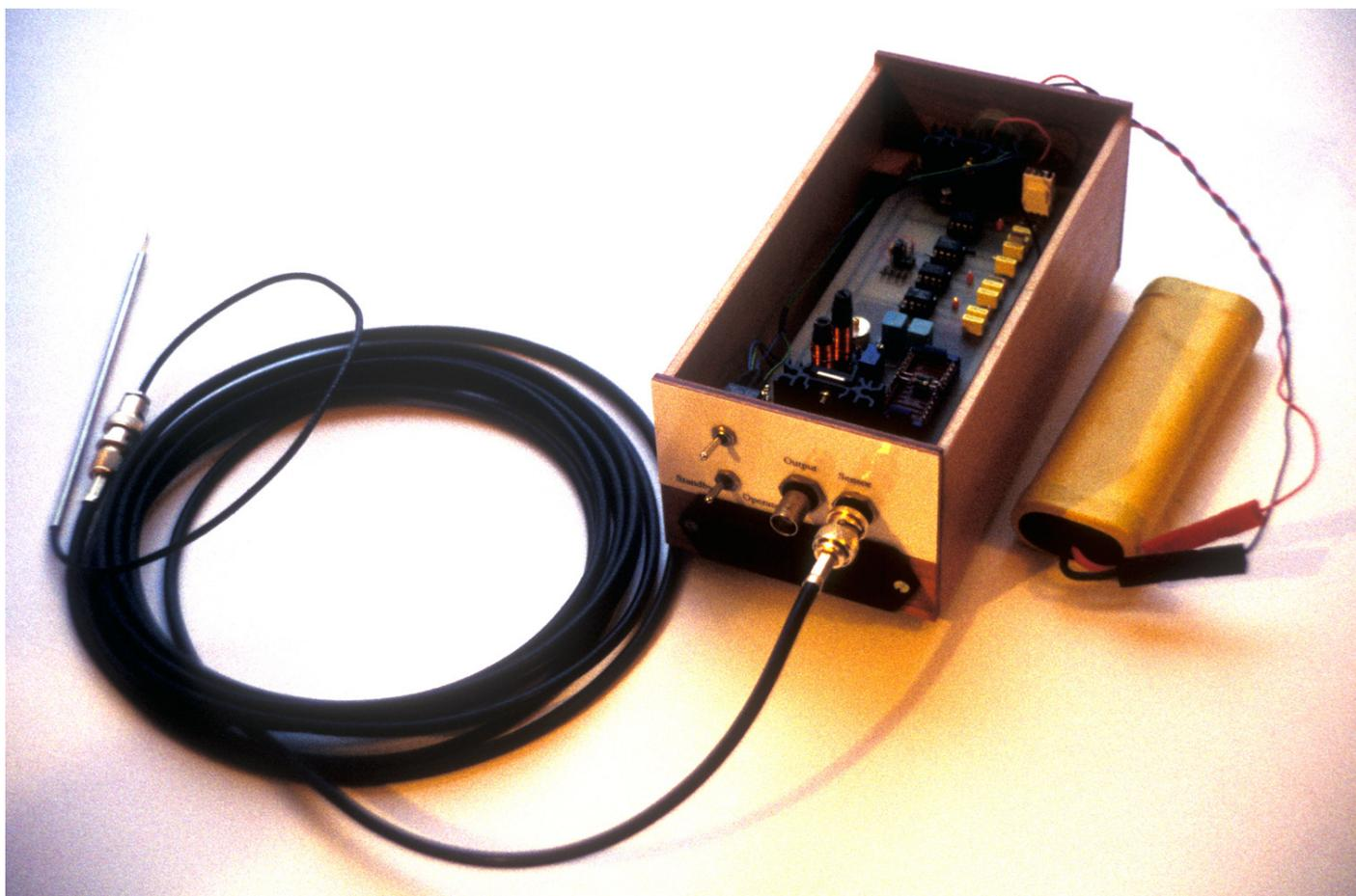
Figure 5. Hot wire anemometer for drag and turbulence measurement. This is described in detail in appendix A.
