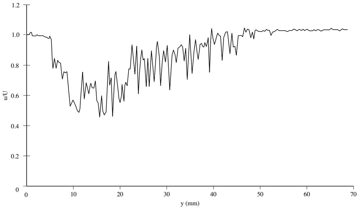
Fig 9.1 Wake profile for  $\alpha = 4$ , rms free stream turb. Intensity = 0.26%, clean wing. To calculate one drag point several such velocity profiles are averaged.
