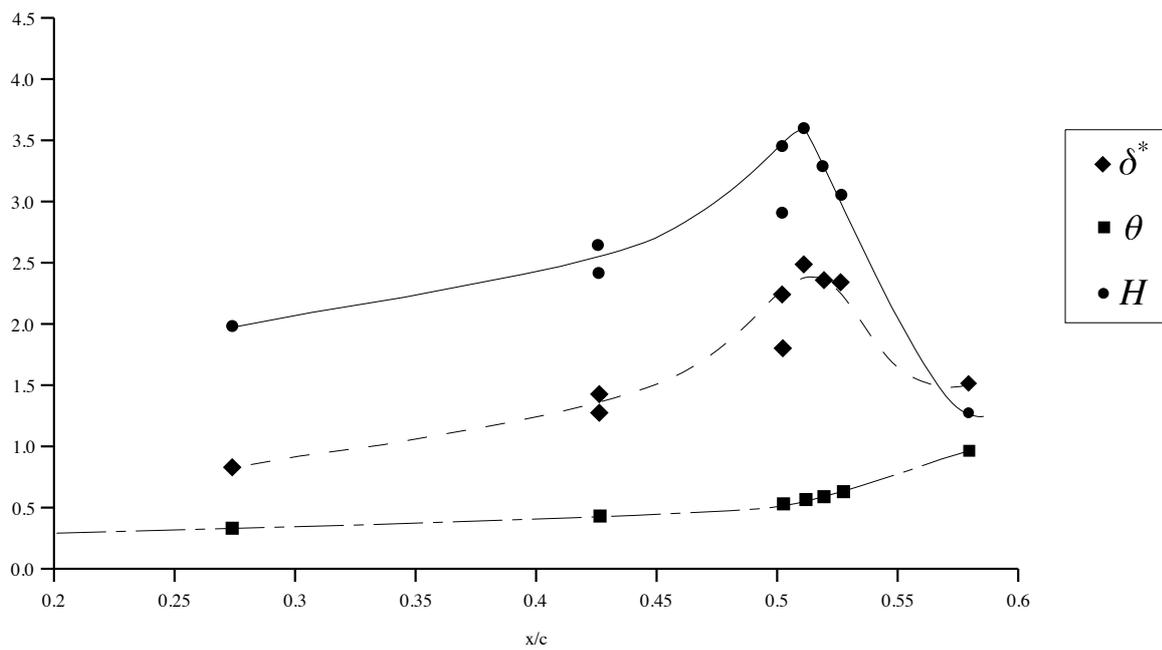
Fig. 8.1 Boundary layer parameters on suction surface at  $\alpha = 0$  degrees
