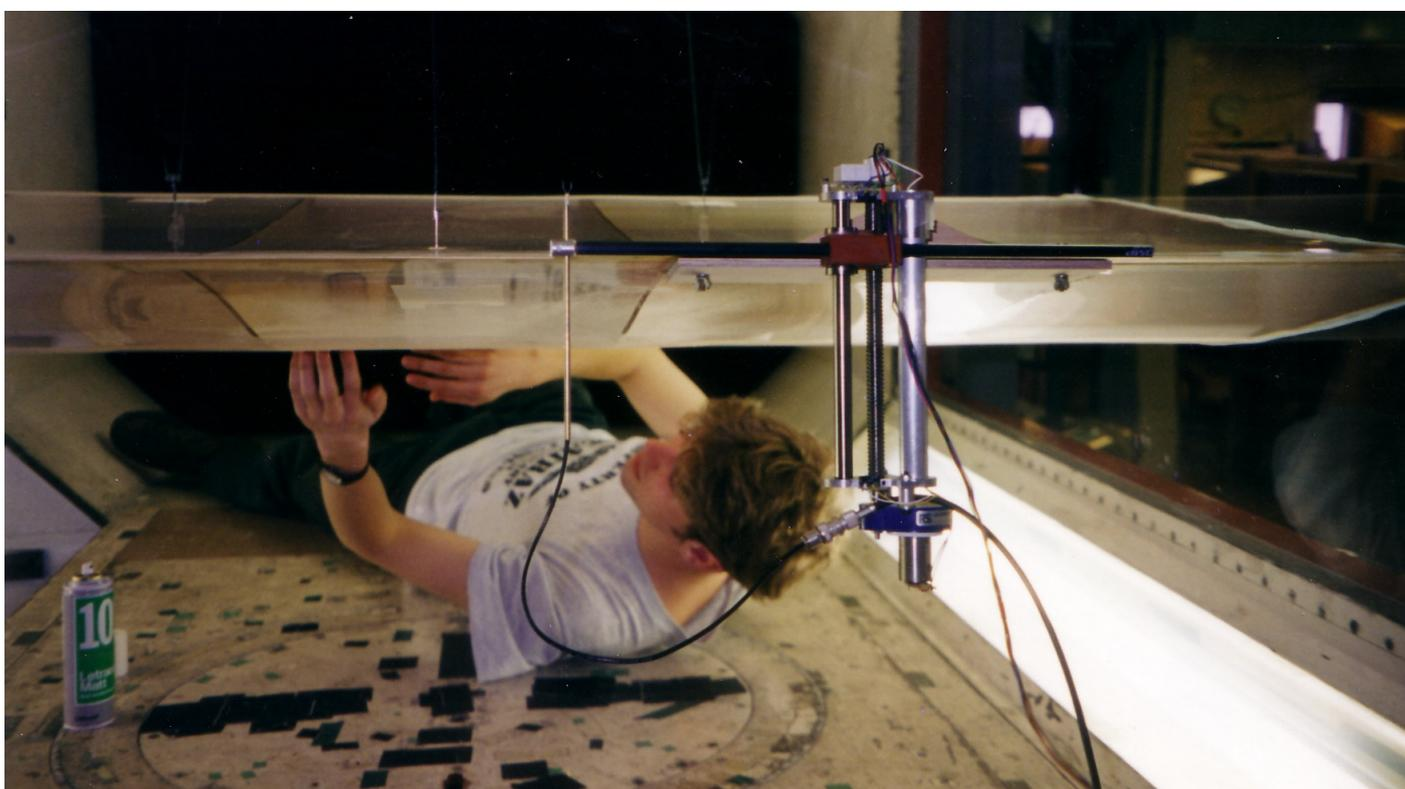
Figure 6. Richard in the Markham wind tunnel with the full sized wing section. The hot wire anemometer wake traverse is mounted on the trailing edge. Micro switches limit the travel of the probe and reverse its direction through a flip flop constructed from relays. A drawing of the traverse with some notes is given in appendix B.
