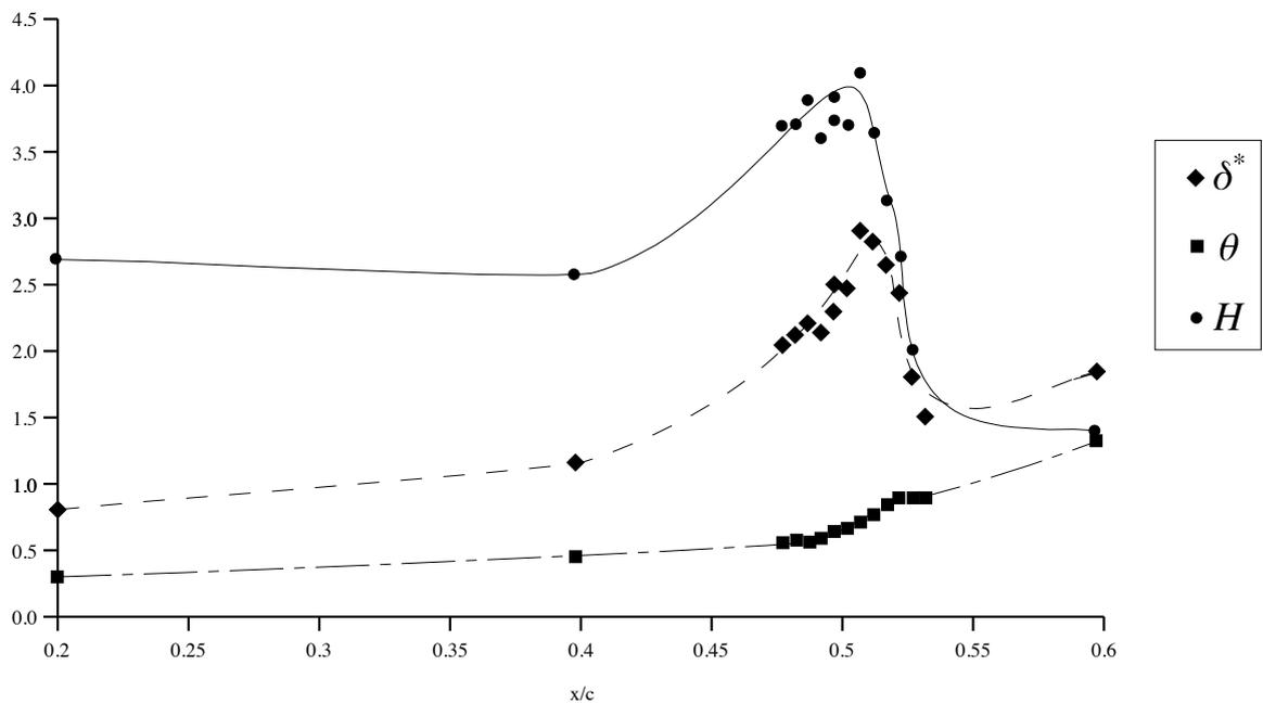
Fig. 8.2 Boundary layer parameters on suction surface at  $\alpha = 4$  degrees
