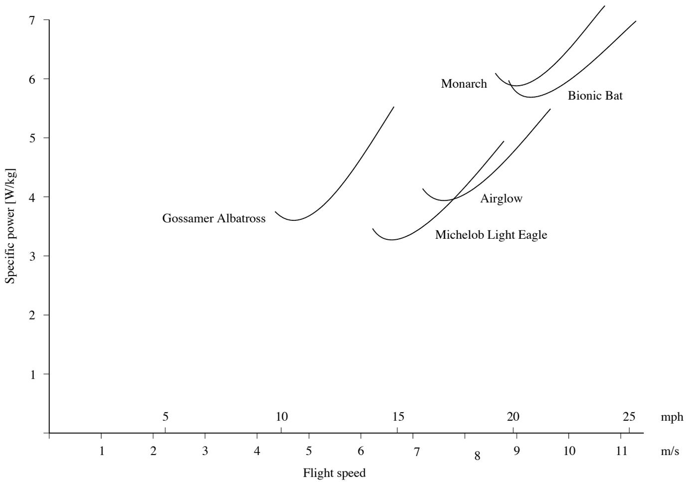
Fig. 2. Power polars for some human powered aircraft
