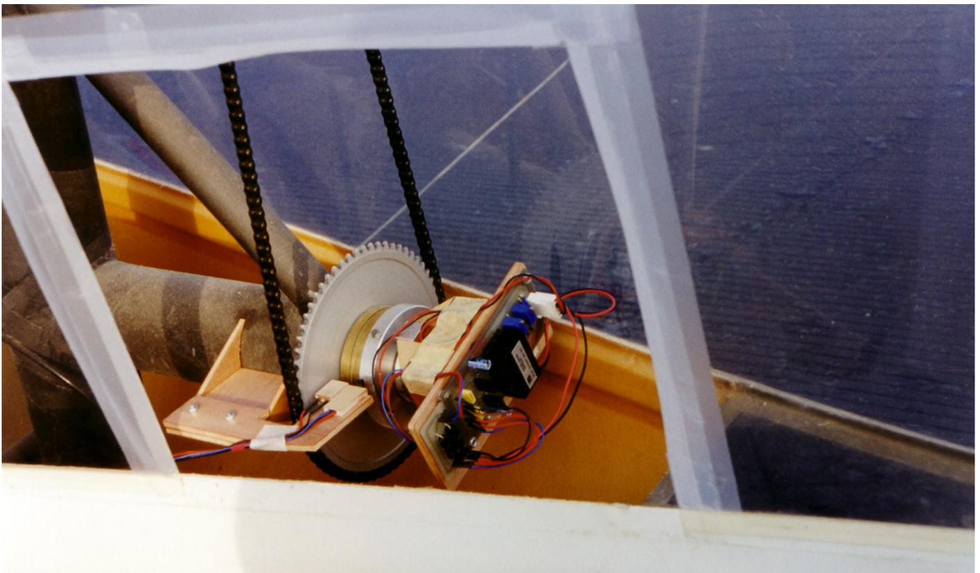
Figure 4. A strain gauged beam at the end of the drive shaft is used to measure torque and hence power input in flight. The voltage signal is sent through slip rings to a data logger. Rotation rate is measured with a hall effect sensor and magnet.
